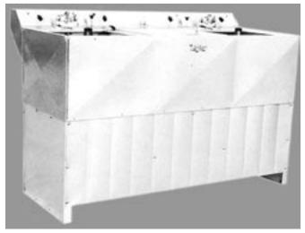
2 wash compartments and 1 rinse-extractor compartment. Capacity: 100-120 lbs. dryweight per hour. Dimensions: length 60", width  $29\frac{1}{2}$ ", height  $40\frac{1}{2}$ ". Weight approximately 460 lbs.
